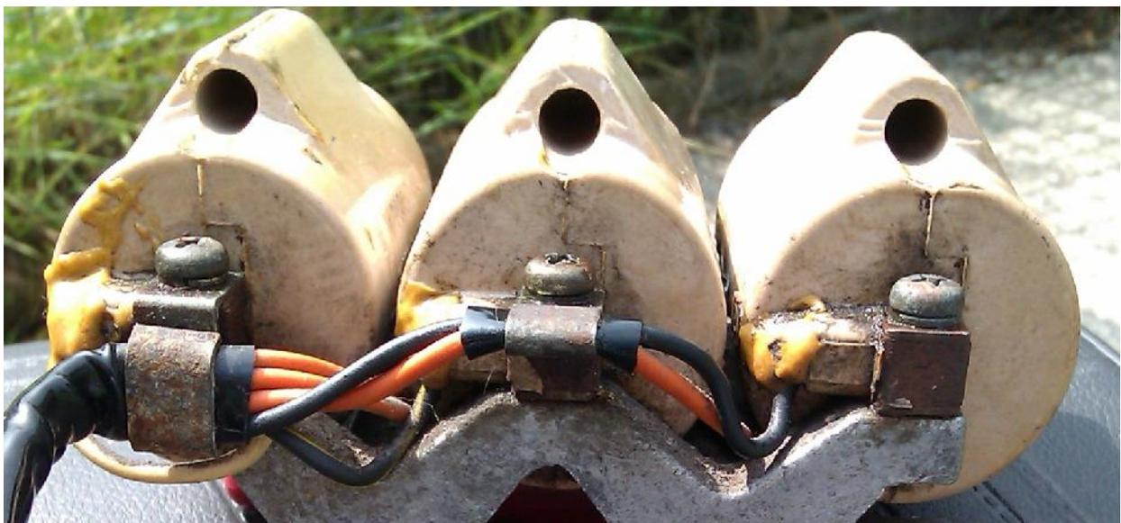
*New leads in place prior to gluing with epoxy resin*
