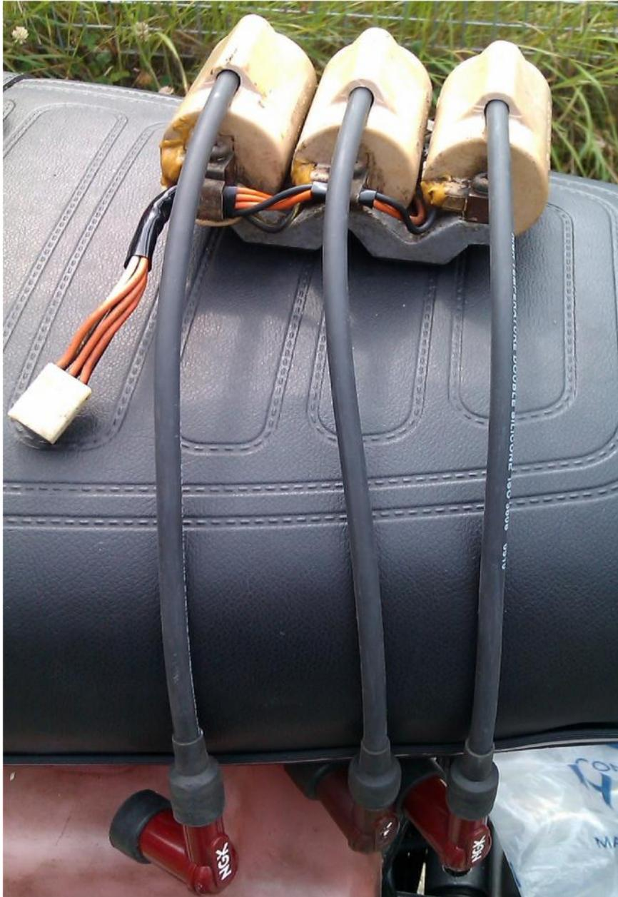
*Epoxy resin set and coils ready to refit*
