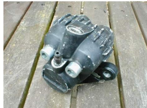
*Calliper taken apart showing damaged rubber seal and "dry" sliding pins*
