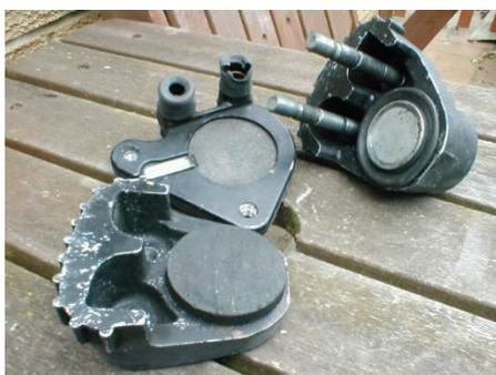
*Piston appears to be in good condition ..... note missing sliding pin "O" rings*
