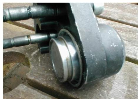
*Piston removed, showing that it is badly pitted and in need of replacement*
